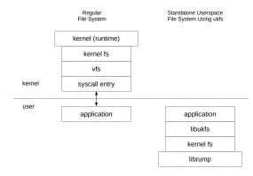
UKFS is a library which uses RUMP. The UKFS interface is based on pathnames and each call is selfcontained for ease of use. This means that it is not necessary to e.g. open a file before reading it. The file system image is mounted internally within the process using UKFS. The kernel mount system call is not used, and the mountpoint is accessible only within the process which is did the mounting.
