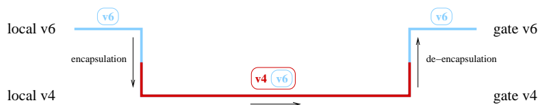
Figure 26-1. A frequently used method for transition is tunneling IPv6 in IPv4 packets
